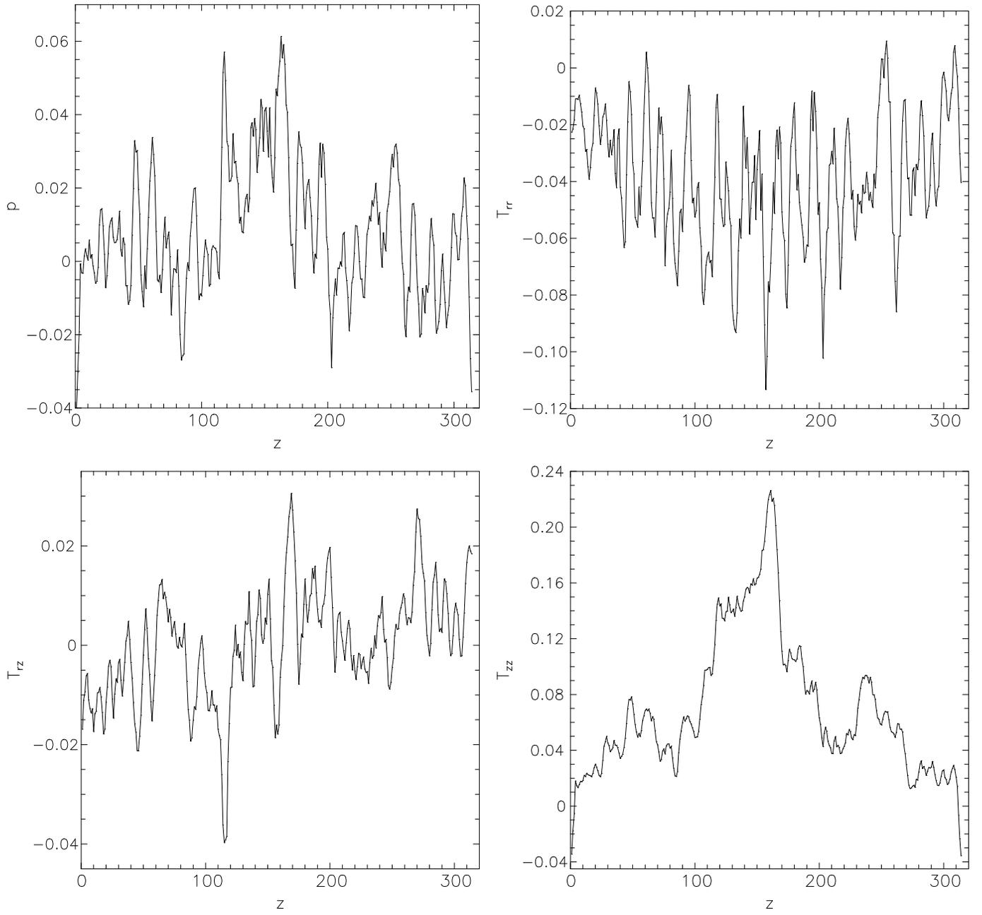
FIG. 7. Stress tensor components *vs.* axial position in the constant velocity deformation of Fig. 1 at time  $2500\tau$ . Clockwise from upper left: pressure ( $p$ ), radial ( $rr$ ), axial ( $zz$ ), and shear ( $rz$ ) stress.
