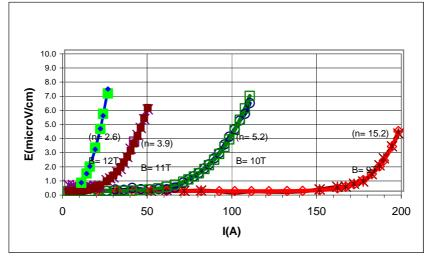
Figure 3 - E(I) characteristics of the sample A , at 4.2 K, in different magnetic fields.
