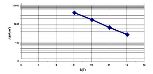
Figure 4 - Critical current density, as function of the magnetic field B, measured by transport method a 4.2 K
