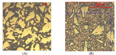
Figure 1 – Optical micrographs of the two examined  $MgB_2$  bulk samples: (A) previous preparation ; (B) present preparation
