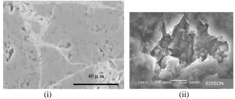
Figure 2 – SEM analysis of the large grain morphology of the sample (A): (i) backscattered electrons image of the large grains ; (ii) an image at higher magnification of an hole inside the large grains reveals a finer grain morphology 2
