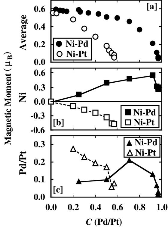
Fig. 1. The experimental (a) average magnetic moment, (b) local magnetic moment at Ni site, plotted with respect to the bulk Ni magnetic moment of  $0.616 \mu_B$ , and (c) local magnetic moment at Pd (Pt) site in Ni-Pd and Ni-Pt alloys
