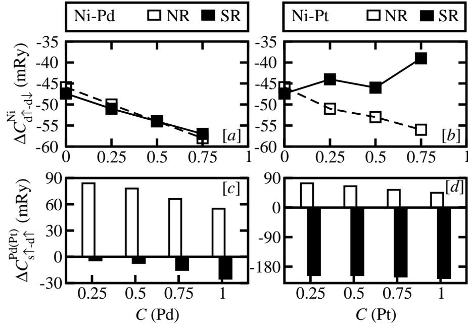
Fig. 4. The non relativistic (NR) and scalar-relativistic (SR) exchange-induced splitting of majority spin and minority spin d-band centers of Ni in (a) NiPd and (b) NiPt alloys. Figures (c) and (d) show the separation between majority spin s and d band centers of (c) Pd in NiPd and (d) Pt in NiPt alloys.
