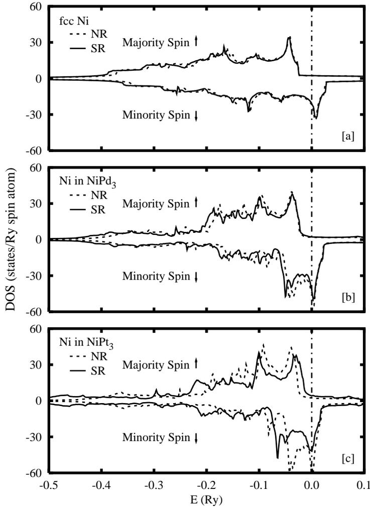
Fig. 3. The spin-polarized densities of states of Ni, calculated non relativistically (NR) and scalar-relativistically (SR), in (a) fcc Ni, (b)  $L_{12}$  NiPd<sub>3</sub>, and (c)  $L_{12}$  NiPt<sub>3</sub>.
