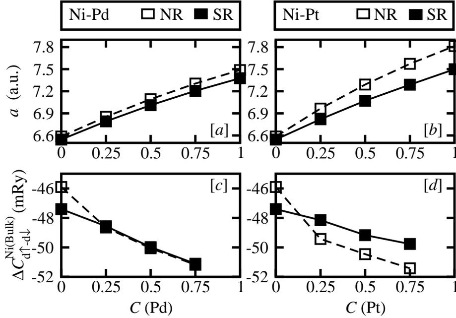
Fig. 5. The non relativistically (NR) and scalar-relativistically (SR) calculated equilibrium lattice constants for (a) Ni-Pd and (b) Ni-Pt alloys. Figures (c) and (d) show the exchange-induced splitting between the majority and minority d band centers in fcc Ni, calculated using the average Wigner-Seitz radii in bulk Ni equal to the radii of the charge neutral Ni atomic spheres in (c) Ni-Pd and (d) Ni-Pt alloys.
