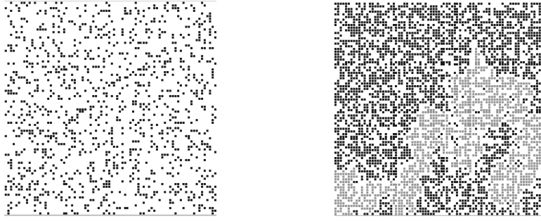
FIG. 2: Typical output 20 of the site percolation algorithm implemented on a two-dimensional square lattice for p < p_c (left panel) and p = p_c (right panel). Occupied sites are marked by a dark square, with those belonging to the percolating cluster having a lighter grayscale, while unoccupied sites are unmarked.
