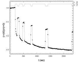
Fig. 1. Normalized resistivity as a function of time after zero field cooling down to T=81.1 K, for polycrystalline  $La_{0.5}Ca_{0.5}Mn_{0.95}Fe_{0.05}O_3$ . The applied field value is H=0.4 T during time intervals of 1, 2, 4, 8 and 16 minutes.
