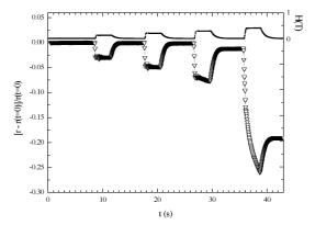
Fig. 2. Normalized resistivity as a function of time after zero field cooling down to T= 94.5 K, for polycrystalline  $La_{0.325}Pr_{0.300}Ca_{0.375}MnO_3$ . Applied field values were H= 0.1, 0.2, 0.3 and 0.4 T for 3 seconds, with time intervals of 6 seconds.
