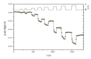
Fig. 3. Normalized resistivity as a function of time after zero field cooling down to T= 91.1 K, for single crystalline  $La_{0.275}Pr_{0.350}Ca_{0.375}MnO_3$ . Applied magnetic field values were H= 0.1, 0.2, 0.3, 0.4, 0.5, 0.6, 0.7 and 0.8 T.
