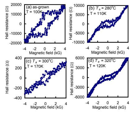
**Figure 4**. Ferromagnetic Hall hyteresis loops of a 0.3 ML Mn  $\delta$ -doped GaAs layer with I-HEMT ( $d_s = 0 \text{ nm}$ ) grown at 300°C; (a) as-grown sample measured at 100K, (b) annealed sample with  $T_a = 280^{\circ}$ C measured at 110K, (c) annealed sample with  $T_a = 300^{\circ}$ C measured at 170K, and (d) annealed sample with  $T_a = 320^{\circ}$ C measured at 120K.
