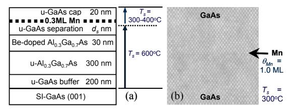
**Figure 1**. (a) Sample structure of a Mn  $\delta$ -doped layer with a selectively doped I-HEMT structure. Holes are supplied into the Mn  $\delta$ -doped GaAs layer from the Be-doped Al<sub>0.3</sub>Ga<sub>0.7</sub>As layer. The GaAs separation layer thickness  $d_s$  was  $0 \sim 10$  nm. (b) High-resolution TEM lattice image of the Mn  $\delta$ -doped GaAs layer at  $\theta_{Mn} = 1.0$  ML grown at  $T_s = 300^{\circ}$ C.
