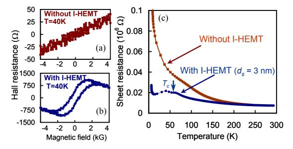
**Figure 2**. (a) and (b) show Hall loops of 0.3 ML Mn  $\delta$ -doped GaAs layers grown at 400°C *without* and *with* I-HEMT ( $d_s = 3$  nm), respectively, indicating a ferromagnetic order in the I-HEMT structure at 40K; (c)  $R_{\text{sheet}} - T$  traces of the samples *without* and *with* I-HEMT, respectively.
