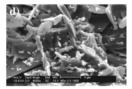
Fig. 1c, d. SEM images of LiBC samples prepared from various flux compositions  $Li_x BC$ . (c) x = 2.0, tube-like inclusions and LiBC platelets; (d) x = 2.0, after heat treatment 1000°C for 20 h.
