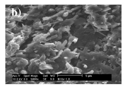
Fig. 1a, b. SEM images of LiBC samples prepared from various flux compositions Li<sub>x</sub>BC.
