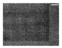
FIG. 3. Vortex decoration of the bottom surface of the thinnest sample investigated, d = 0.5 m. It shows a complete square symmetry of the whole vortex structure beneath the periodic 2D square pattern in the top surface (dark area). The scale bar corresponds to 5 m.
