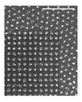
FIG.1. Vortex decoration of the top surface of a sample with commensurate square magnetic pattern for a eld of 30.2 G auss at 4.1 K. The Fe dots of the periodic structure are 260 nm in diameter and 60 nm in height. The dark area indicates the region where a periodic 2D square pattern was generated. The Fe dots positions are depicted with white circles. The scale bar corresponds to 5 m.
