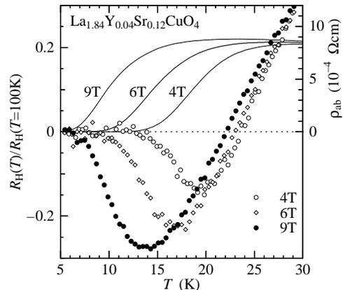
FIG. 3: The temperature dependence of the Hall coefficient and the resistivity of  $\text{La}_{1.84}\text{Y}_{0.04}\text{Sr}_{0.12}\text{CuO}_4$  in 4 T, 6 T and 9 T. Marks and solid lines denote the Hall coefficient and the resistivity, respectively.
