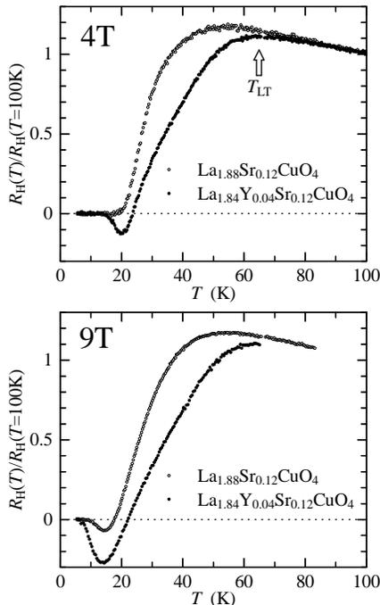
FIG. 2: The temperature dependence of the Hall coefficient of  $\text{La}_{1.88-y}\text{Y}_y\text{Sr}_{0.12}\text{CuO}_4$  ( $y = 0$ : open circles,  $y = 0.04$ : closed circles) in 4 T and 9 T. The arrow in the figure indicates the structural phase transition temperature to the TLT phase in the case of  $y = 0.04$ .
