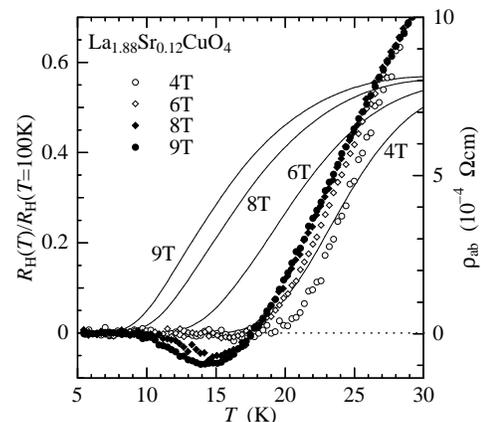
FIG. 4: The temperature dependence of the Hall coefficient and the resistivity of  $\text{La}_{1.88}\text{Sr}_{0.12}\text{CuO}_4$  in 4 T, 6 T, 8 T and 9 T. Marks and solid lines denote the Hall coefficient and the resistivity, respectively.
