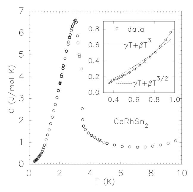
Fig.3. Specific heat of  $CeRhSn_2$ . The inset shows fits of the experimental data as mentioned in the text.
