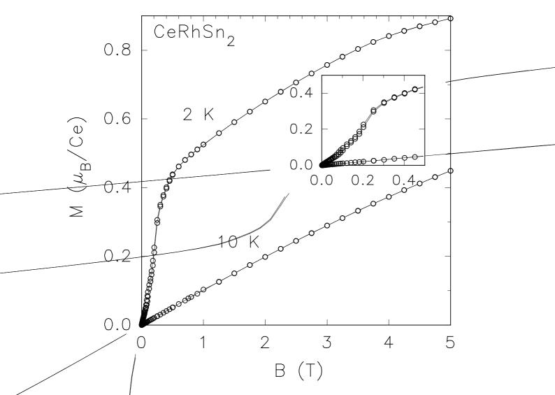
Fig.2. Magnetization as a function of field at 2 K and 10 K.
