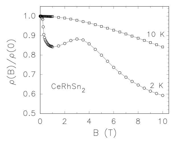
Fig.5. Normalized magnetoresistance as a function of field for  $CeRhSn_2$ .
