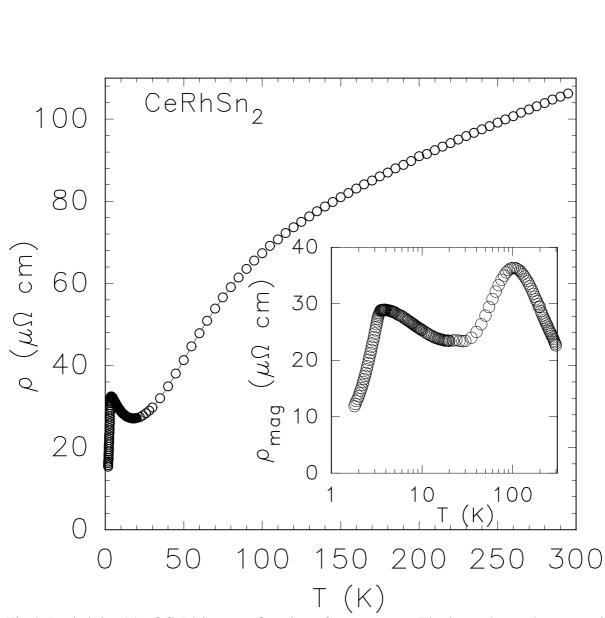
Fig.4. Resistivity ( $\rho$ ) of CeRhSn<sub>2</sub> as a function of temperature. The inset shows the magnetic part of the resisvity ( $\rho_{mag}$ ).
