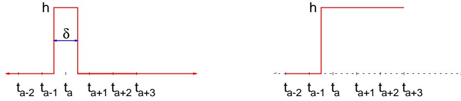
Figure 8: Left: an instantaneous perturbation applied at t_a . Right: a step perturbation applied at t_a and held constant for all subsequent times.
