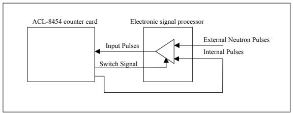
Figure 5: Schematic of switching between external and internal pulses.
