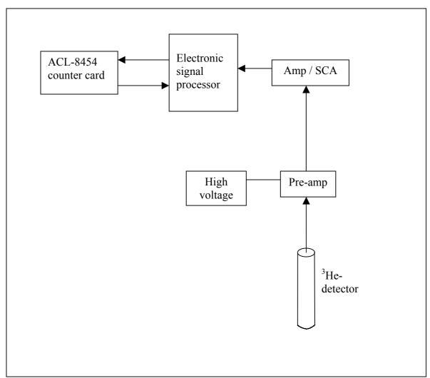
Figure 2: Schematic of detection hardware (For simplicity only one detector is shown).
