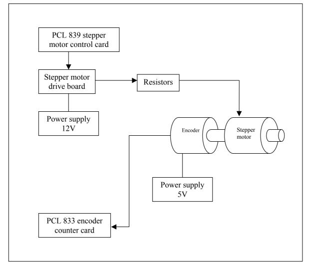
Figure 1: Schematic of motion control hardware (For simplicity only one stepper motor is shown).
