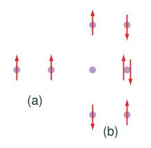
FIG. 2 M otion of the two ferrom agnetically aligned spins in (a) is prohibited by the Pauli principle. In contrast, the antiferrom agnetically aligned spins at the top and bottom in (b) can access a high energy interm ediate state (shown in the middle of (b)) and so undergo an exchange process.
