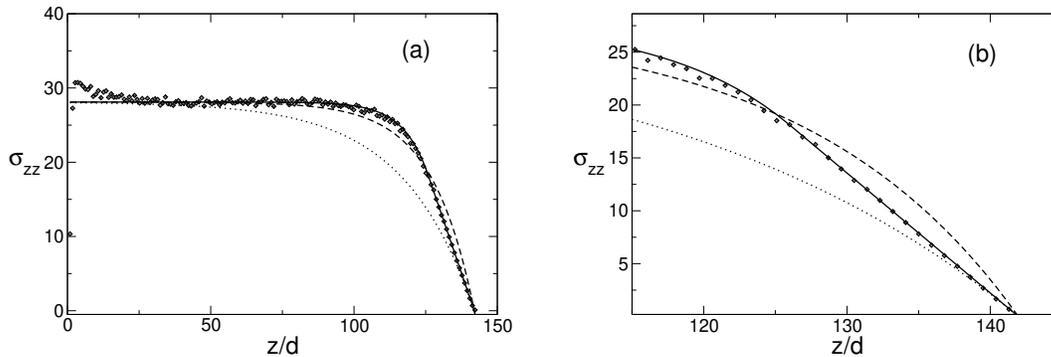
FIG. 6: Vertical stress  $\sigma_{zz}$  in units of  $m g d^2$  for  $N = 50000$  using method S2. The data is represented by the diamonds. The dotted line is a fit to the Janssen expression with  $l = 1$ , Eq. 4. The dashed line is a fit to the modified Janssen expression with  $l \ll 1$ . The solid line is a fit to the two parameter theory, Eq. 5. (b) is a blow up of the turnover region on the right side of (a).
