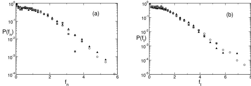
FIG. 9: Distribution of normal  $f_n$  and tangential  $f_t$  contact forces for a packing of 50,000 particles generated using method P1. Bulk forces are represented as open circles, forces between particles and side wall are represented as filled-in triangles, and forces between particles and the flat base are represented as filled-in squares. All forces exhibit the same quasi-exponential tails.
