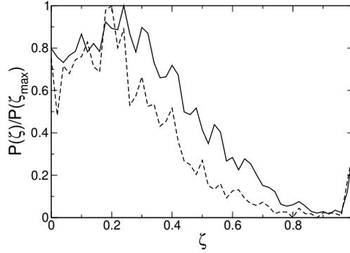
FIG. 11: Probability distributions  $P(\zeta)$  at the side wall in the linear hydrostatic region at the top of the packing with  $\mu_w = 0.5$ , each normalized by its maximum value  $P(\zeta_{\max})$ .  $F_t = \mu_w F_n$ . The solid line is the data for method S2 and the dashed line the data for method P1. In contrast to the behavior in the height-independent pressure region, the forces at the walls are far from the Coulomb failure criterion in all cases.
