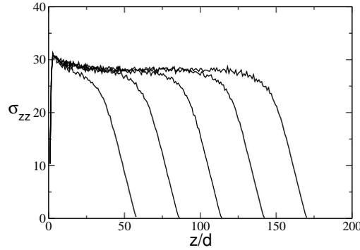
FIG. 5: Vertical stress  $\sigma_{zz}$  in units of  $m g d^2$  for  $N = 20000$  to  $60000$  packings with a rough base, using  $\mu_w = 0.5$  and  $R = 10d$  for method S2. Data for each value of  $N$  is averaged over 6 runs.
