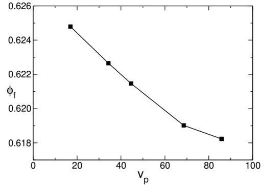
FIG . 3: Final average packing fraction  $\phi_f$  as a function of pouring rate  $v_p$  (in units of  $1=$  ). Results are for packings of 50;000 particles with  $R = 10d$  poured from a height of  $180d$  with method P1. The line is a guide to the eye. Slower pour rates create denser packings.
