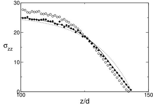
FIG. 7: Vertical stress  $\sigma_{zz}$  in the top part of  $N = 50000$  packings, with  $\mu_w = 2$  (diamonds) and  $\mu_w = 0.5$  (open circles), both using method S2. The dotted line is a fit to the  $\mu_w = 2$  data with the modified Janssen formula with  $\beta = 1$  and the straight line is a fit to the same with the two-parameter Vanel-Clement formula.
