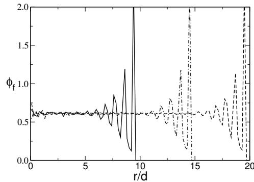
FIG . 4: Final volume fraction  $\phi_f$  of packings as a function of radius for packings of  $N = 50;000$  and  $R = 10$ ,  $N = 82;000$  and  $R = 15$ , and  $N = 144;000$  and  $R = 20$  using method S2. The effects of the wall penetrate about  $4d$  in each case.
