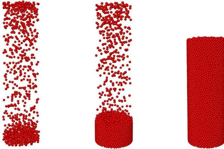
FIG. 1: Formation of a packing of  $N = 20,000$  spheres in a cylindrical container of radius  $10d$  onto a flat base. The packing is constructed by pouring using method P1 from a height of  $70d$ . The configurations shown are for early, intermediate and late times. The final static pile has  $\phi_f = 0.62$ .
