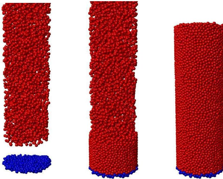
FIG. 2: Lower portion of the packing of  $N = 20,000$  spheres in a cylindrical container of radius  $R = 10d$ . The packing is supported by a rough bed (darker particles) and is constructed by sedimentation using method S2. The three configurations shown are the initial configurations with volume fraction  $\phi_i = 0.13$ , an intermediate one, and the final static pile with  $\phi_f = 0.60$ .
