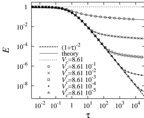
FIG. 2: Energy  $E$  plotted against time  $\tau$  for a simulation with  $N = 19683$  particles, density  $\nu = 0.08245$ , coefficient of restitution  $r_0 = 0.99$  and different  $V_c$  as given in the inset. The symbols are simulations and the lines give the solution of Eqs. (2,3), using Eqs. (4,5).
