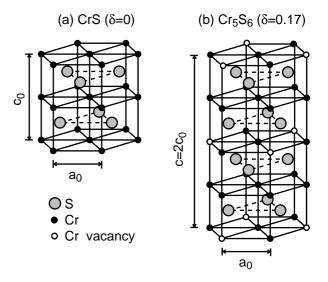
Figure 1. Crystal structures of (a) CrS and (b) Cr<sub>5</sub>S<sub>6</sub>.
