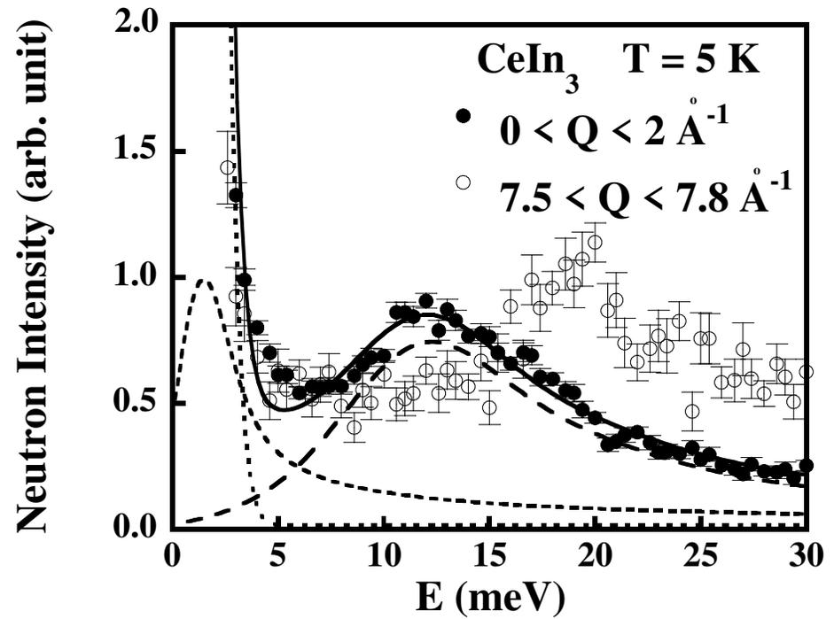
Figure 2. Energy scans at different wavevectors obtained on the MARI spectrometer using an incident energy of 60.3 meV at  $T = 5$  K. The long dashed, short dashed, and dotted lines show the CF, QE, and incoherent contributions of the small  $Q$  spectrum, respectively, while the solid line shows the total.
