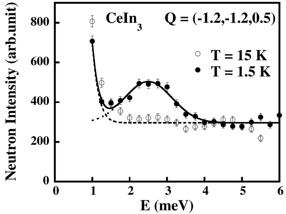
Figure 3. Energy scans at  $Q = (-1.2, -1.2, 0.5)$  for temperatures of  $T = 1.5$  and  $15$  K obtained on the IN22 spectrometer using a final energy of  $14.7$  meV.
