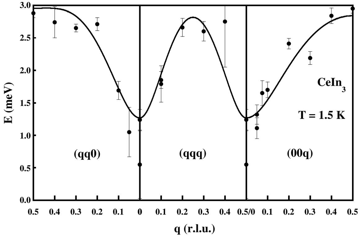
Figure 4. Spin-wave dispersion of  $\text{CeIn}_3$  along the three main directions  $(0;0;q)$ ,  $(q;q;0)$  and  $(q;q;q)$  at  $T = 1.5 \text{ K}$ , obtained on the IN22 spectrometer using a neutron energy of  $14.7 \text{ meV}$ . The solid line is a fit obtained using the molecular-field random-phase approximation.
