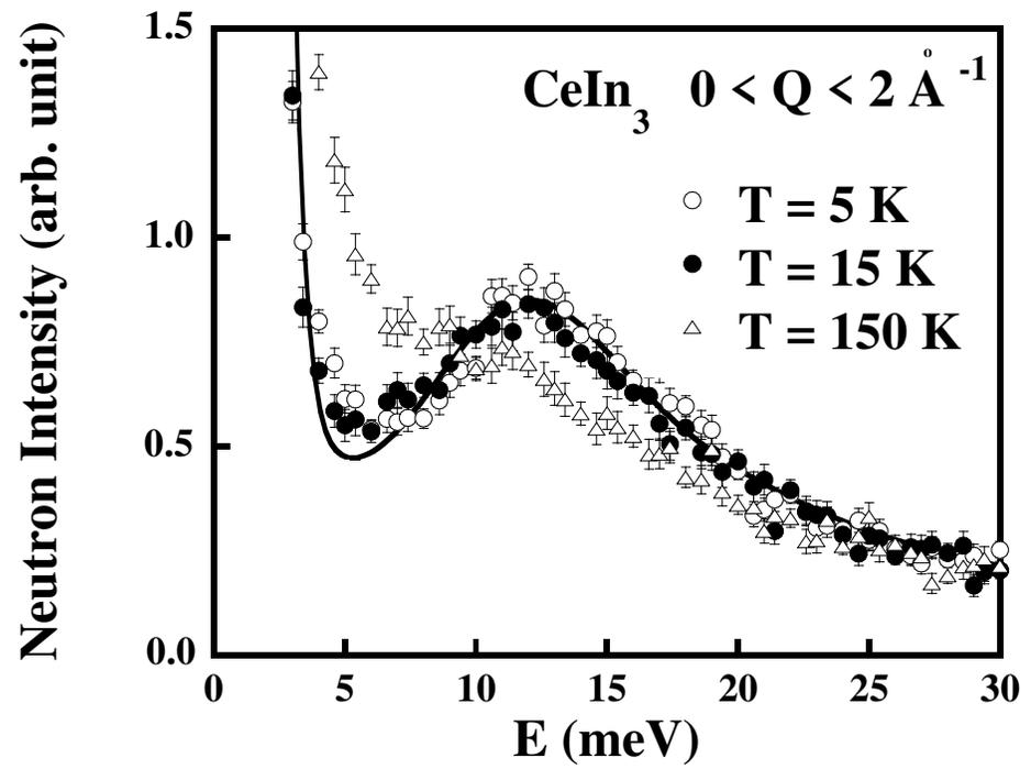
Figure 1. Energy scans at different temperatures obtained on MARI spectrometer using an incident energy of 60.3 meV and integrating over  $Q$  values between 0 and  $2 \text{ \AA}^{-1}$ . The solid line shows the total fit for  $T = 5 \text{ K}$ .
