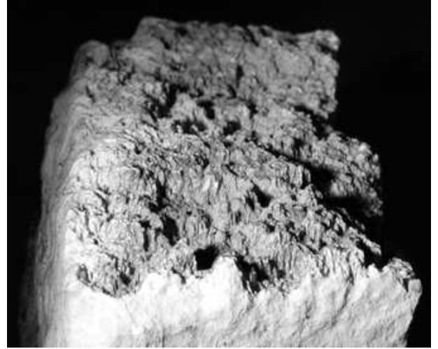
FIG. 1: Picture of the stylolite surface that has developed in a limestone from Juras Mountains (France). Magnitude of the peaks are typically of the order of 2 mm. The width of the sample is 4 cm.
