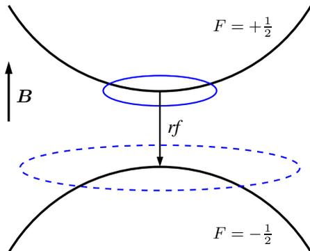
FIG. 1: Exponential expansion of a two-component Bose-Einstein condensate with effective spin  $F = 1/2$ , to create a de Sitter quasiparticle universe close to its center. The trapping potential is inverted by applying a radio frequency ( $rf$ ) pulse, which transfers the atoms to their untrapped hyperfine state.
