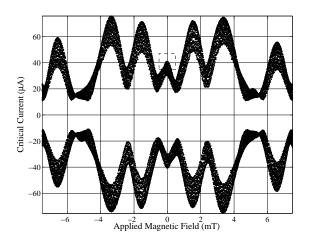
FIG. 2: Critical current as a function of magnetic eld at 4.2K. The dashed box indicates the area plotted in g. 3a.
