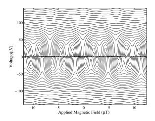
FIG.4: Voltage modulation as a function of applied magnetic eld for the SQUID whose  $I_c$  B is shown in g. 3a. The pattern is again inversion symmetric. Note the sign change at 100 V which we believe is due to a LC-resonance in the SQUID loop.
