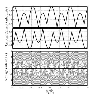
FIG.1: The results of simulations of the  $I_c \ x$  and V x dependence for a dc-SQUID with  $I_{c1}^{\rm I} = 1$ ,  $I_{c2}^{\rm I} = 0$ :1,  $I_{c1}^{\rm II} = 0.2$  and  $I_{c2}^{\rm II} = 0.4$  (arb. units). The dimenstructures correspond to bias currents in the range I =  $I_{c1}^{\rm I}$  to I =  $5I_{c1}^{\rm I}$  W e assume L = 0 and  $G_1 = G_2$ .
