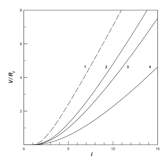
FIG. 2. The current–voltage characteristics at different values of g-parameter for Euclidean clusters (D = 1, dotted line), and for the clusters of the most fractal boundaries (D = 2, solid line). Curve (1) corresponds to the case of D = 1, g = 0; curve (2) of D = 2, g = 0.5; curve (3) of D = 2, g = 0; curve (4) of D = 2, g = -0.5.
