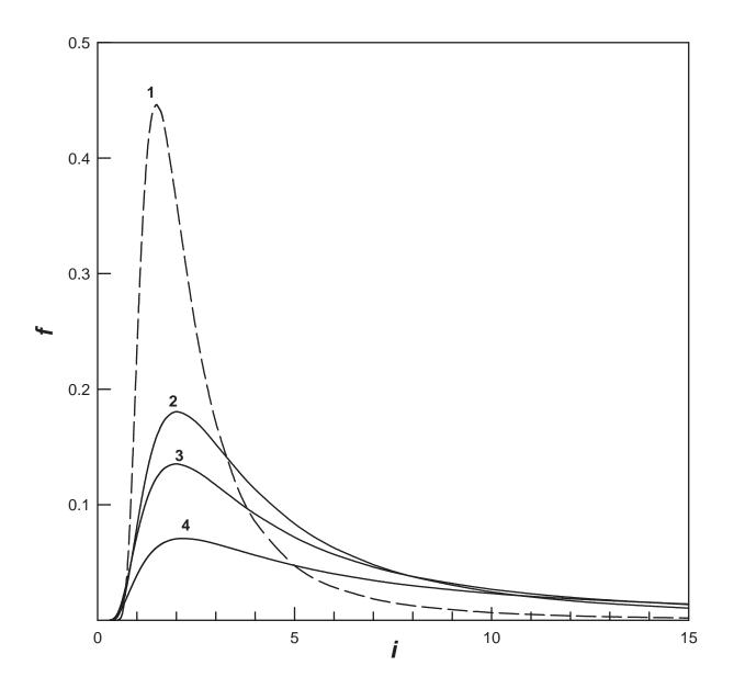
FIG. 1. Influence of the fractal dimension D and g-parameter of gamma-distribution on the distribution of critical currents. The dotted line is drawn for the Euclidean clusters (D = 1); and the solid lines for the clusters with the most fractal boundaries (D = 2). Curve (1) corresponds to the case of D = 1, g = 0; curve (2) of D = 2, g = 0.5; curve (3) of D = 2, g = 0; curve (4) of D = 2, g = -0.5.
