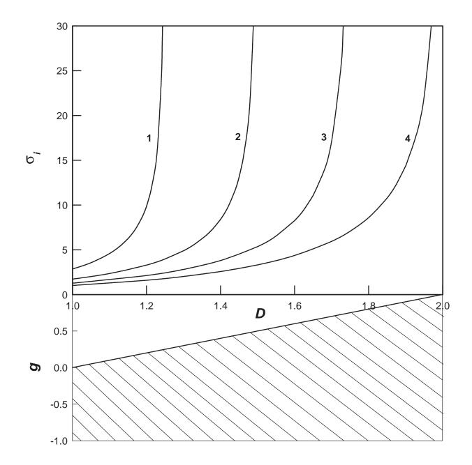
FIG. 3. Influence of the fractal dimension of the cluster boundary on the standard deviation of critical currents at different values of g-parameter. Curve (1) corresponds to the case of g = 0.25; curve (2) of g = 0.5; curve (3) of g = 0.75; curve (4) of g = 1. The region of giant dispersion of the critical current ( $D \ge g + 1$ ) is shown by hatching.
