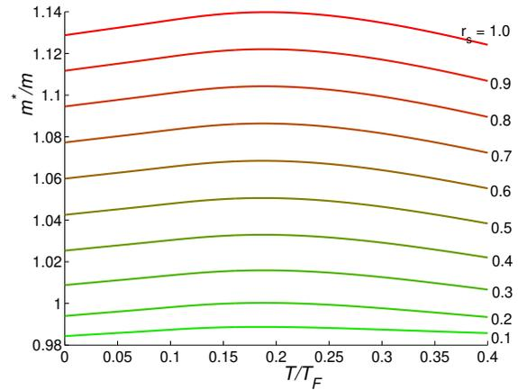
FIG. 5: Calculated 2D effective mass as a function of  $T=T_F$  for different low  $r_s$  values:  $r_s = 1 \dots 0.1$  from top to bottom.
