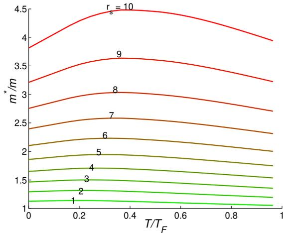
FIG. 4: Calculated 2D effective mass as a function of  $T=T_F$  for different high  $r_s$  values:  $r_s = 10 \dots 1$  from top to bottom. Note that  $T_F / r_s^2$ , making the absolute temperature scale lower for higher  $r_s$  values.
