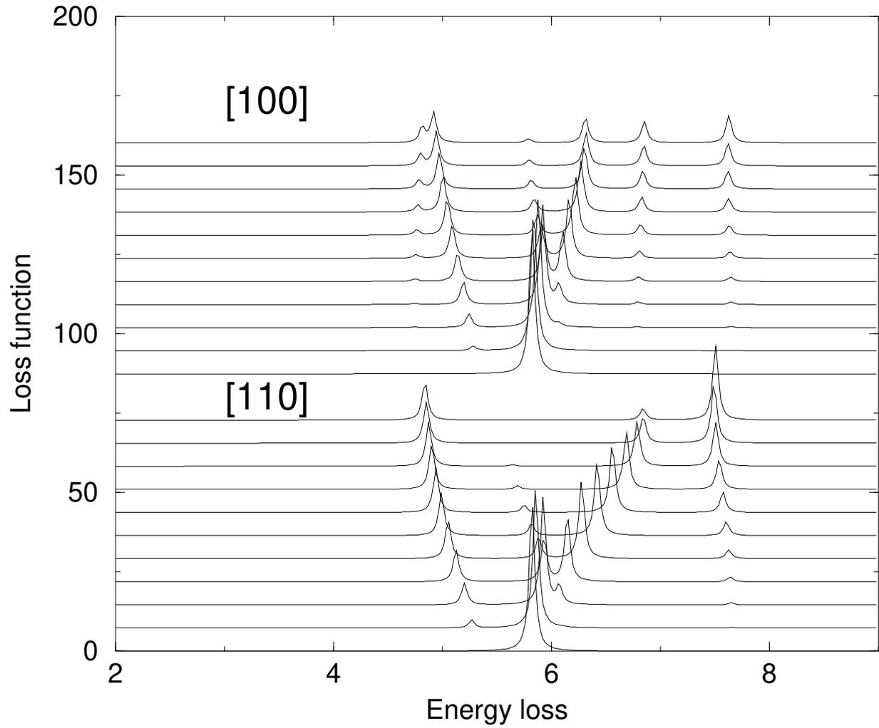
FIG. 2: The loss function  $L(q;!) = \text{Im} \epsilon^{-1}(q;!) \text{ multiplied by } [\epsilon_1(0)]^2$  in order to have approximately the same normalization as  $\epsilon_2(q;!)$  for the same parameters as in Fig. 1 and under the assumption that  $\epsilon(q;! = 0) = \epsilon(q = 0;! = 0) = 4.83$ .
