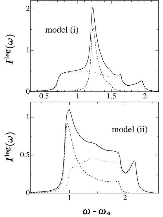
FIG. 4: The optical-absorption spectra for E k legs in model (i) and model (ii) for  $N = 28$ . The dashed lines and dotted lines represent the spectra from the  $q_y = 0$  mode and  $q_y = \pi$  mode, respectively, and the solid lines indicate their sum.
