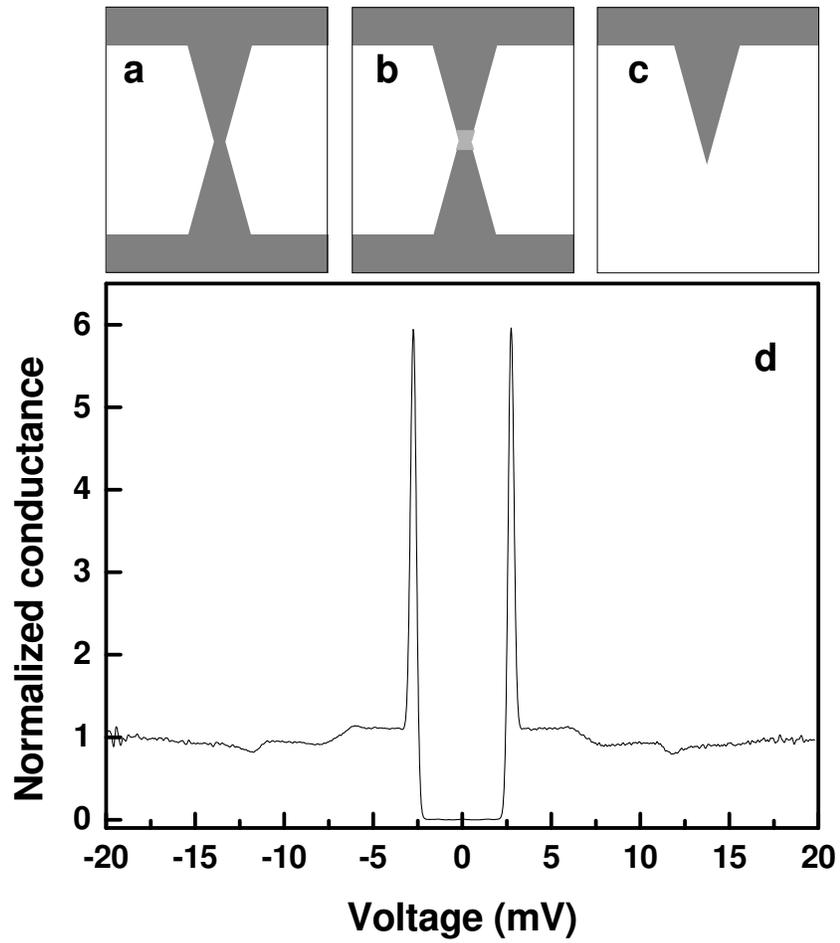
FIG. 1: The three main structures described in the text are shown schematically: a) nanobridge (NB), b) neck, and c) nanotip (NT). In d) we show a typical experimental conductance curve obtained in tunneling regime, in zero magnetic field, at 1.5 K. (tunnel resistance is  $R_N = 1.5 \text{ M}\Omega$ ).
