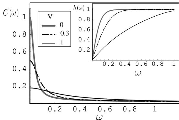
FIG. 3: Voltage-dependent spin correlator  $C(\omega)$  calculated for a sequence of voltages  $V = 0, 0.3, 1$  at a temperature  $T = 0.05$ . Here  $\alpha = 1$  and  $\bar{J} = 0.2$ . Inset, fluctuation-dissipation function  $h(\omega)$  for the same sequence of voltages.
