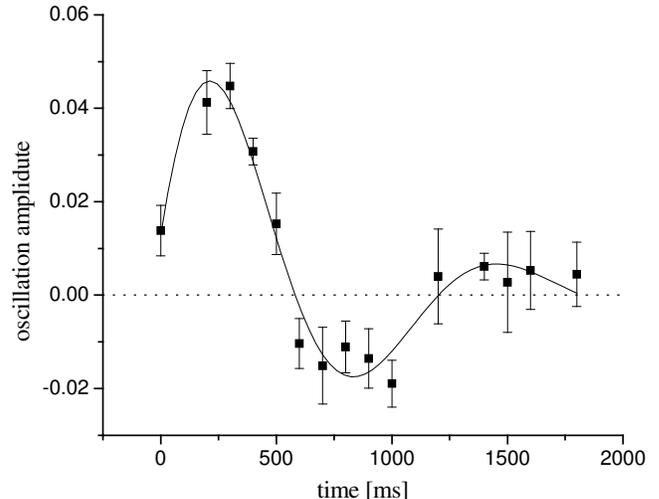
FIG. 2. Measured oscillation amplitude for a typical excitation  $\Omega=0.92$  and  $2.2 \times 10^6$  atoms. Fit is to a sinewave times an exponential decay and yields a frequency of 0.85 Hz and a Q of 3. The oscillation amplitude is expressed as the average amplitude of the sinewave fits to the vortex oscillation in units of the radial Thomas-Fermi radius (roughly the azimuthal displacement of a vortex a distance  $0.33 R_\rho$  from the condensate center). Both values are in expansion.
