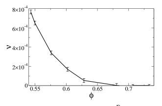
FIG.4: Equilibrium anisotropy  $(1 \frac{c}{a} = \frac{p}{\frac{b}{3}})$  for the hcp hard sphere crystal as a function of packing fraction.
