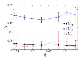
FIG.2: Relative di erence  $j_{ab}^{0fcc} C_{ab}^{0hcp} j C_{ab}^{0fcc}$  between fcc and hcp  $C_{11}^{0}$ ,  $C_{12}^{0}$  and  $C_{13}^{0}$  elastic constants as a function of packing fraction . The results shown were obtained in simulations of a system of 216 particles, with c=a = 8=3. The curves only serve as guides to the eye.
