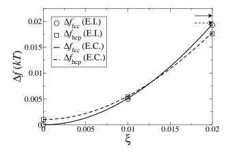
FIG. 3: Variation of the fcc and hcp free energy with deform ation (see Eq. 4). The symbols indicate the results of E instein free energy calculations (see text). The continuous curves were computed on basis of the calculated second and third order elastic constants. The error bars of the E instein free-energy calculations are about one sixth the size of the symbols. The two horizontal arrows show the predictions for f obtained by neglecting the third-order elastic constants.
