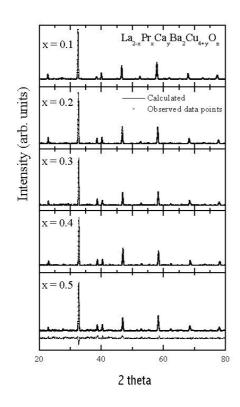
Fig. 1. XRD Rietveld fitted pattern for all the samples. The open circles represent data points, and the line passing through them shows calculated pattern. The difference between observed and calculated pattern is shown for x = 0.5 sample
