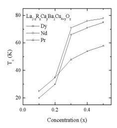
Fig. 4. Variation in  $T_c$  with increasing x, for R = Nd, Dy and Pr in  $La_{2.x}R_xCa_yBa_2Cu_{4+y}O_z$
