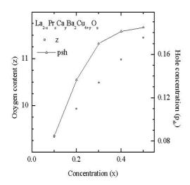
Fig. 5. Change in oxygen content and hole concentration in sheets  $(p_{sh})$ .
