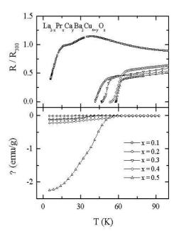
Fig. 3. Transition temperatures for  $La_{2-x}Pr_xCa_yBa_2Cu_{4+y}O_z$  compounds determined by resistivity and susceptibility as a function of temperature.
