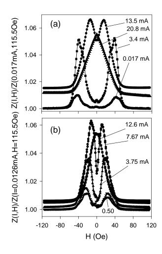
Fig. 3. Normalized GMI Z/Z<sub>s</sub>, where the saturated value at small current is  $Z_s = Z$  (I = 0.02 mA, H = 115.5 Oe), for sample Co<sub>75</sub>Si<sub>10</sub>B<sub>15</sub> at 1 MHz, at different driving current amplitudes; (a) as-cast, (b) after annealing by ac current.
