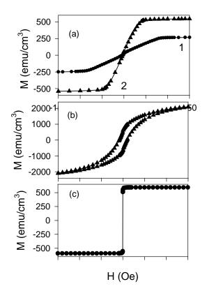
Fig. 1. Axial hysteresis loops for samples with compositions  $Co_{75}Si_{10}B_{15}$  (a),  $Co_{68.2}Mn_{6.8}Si_{10}B_{15}$  (b) and  $Co_{68}Mn_7Si_{10}B_{15}$  (c). In panel (a) curve 1 is the hysteresis loop for as-cast amorphous wire, and curve 2 is for the same sample after annealing by ac current of 50 mA for 0.5 hours.
