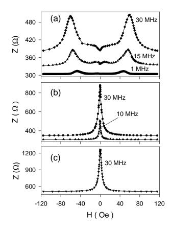
Fig. 2. GMI for samples of  $Co_{75}Si_{10}B_{15}$  (a),  $Co_{68.2}Mn_{6.8}Si_{10}B_{15}$  (b) and  $Co_{68}Mn_7Si_{10}B_{15}$  (c), at a driving current of 2.5 mA. The values of the current frequency are shown.
