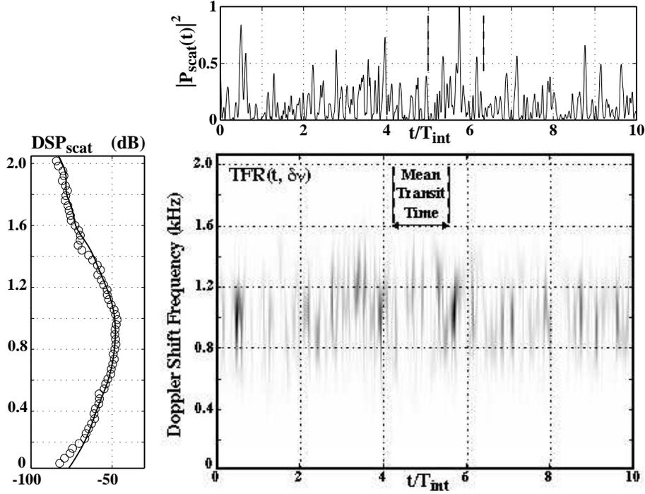
Figure 9. Time-Frequency Analysis of  $z_{scat}(t)$  in the LEGI air jet flow ( $R_\lambda \simeq 785$ ). Center :  $TFD_z(t, \nu)$ , Left : PSD marginal (o) and averaged PSD (-), Top : instantaneous power marginal
