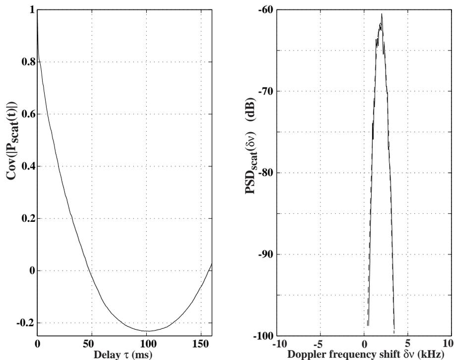
Figure 13. Normalized Covariance  $C_{\rho\rho}(\tau)$  of  $\rho_{scat}(t)$  (left) and  $PSD_{scat}(\delta\nu)$  (right) of the acoustic pressure scattered by soap bubbles in the LEGI turbulent jet flow at  $R_\lambda \simeq 500$ .
