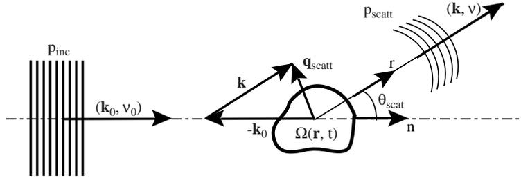
Figure 1. Acoustic Scattering by a Vorticity Distribution
