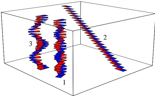
FIG. 2: (Color online) Illustration of DNA geometry for a diameter of  $d = 16\text{\AA}$ : (1) Twisted ladder with  $Sl = Sh = 0$ ,  $Ri = 3.3\text{\AA}$ ,  $Tw \approx 2\pi/10$ , (2) Skewed ladder with  $Tw = Sh = 0$ ,  $Ri = 3.4\text{\AA}$ ,  $Sl \approx 5.0\text{\AA}$ , (3) Helix with  $Tw = 2\pi/12$ ,  $Ri = 3.4\text{\AA}$ ,  $Sl \approx 2.7\text{\AA}$ ,  $Sh \approx 1.6\text{\AA}$ .
