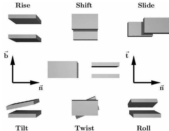
FIG. 1: (Color online) Illustration of all six base-pair parameters and the corresponding coordinate system.
