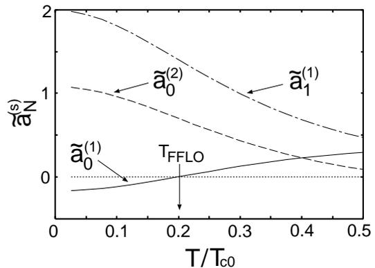
FIG. 7: Temperature dependences of  $\tilde{a}_0^{(1)}$  and  $\tilde{a}_0^{(2)}$  on  $H_{c2}(T)$  and near  $T_{\text{FFLO}}$ , where  $\tilde{a}_0^{(s)} = a_0^{(s)}/\tau_H^{2s}$  ( $s = 1, 2$ ), and the pure limit was assumed. The corresponding curve of  $\tilde{a}_1^{(1)} = a_1^{(1)}/\tau_H^2$  is also shown for a convenience.
