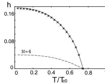
FIG. 1: Comparison between  $H_{c2}(T)$ -curves for  $(2\pi T_{c0}\tau)^{-1} = 0.1$  determined from  $a_0(0) = 0$  by neglecting (crossed symbols) and including (solid curve) the impurity-ladder vertex correction. The dashed curve is the line on which  $a_d(0) = 0$ , and  $h = H/H_{c2}^{\text{orb}}(0)$ .
