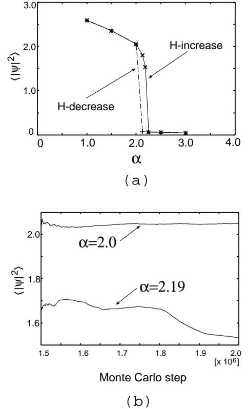
FIG. 13: (a) Numerical data, similar to Fig.11, for  $|\beta| = 3.5$ . (b) The history of  $\langle |\Psi|^2 \rangle$  at  $\alpha = 2.0$  and  $\alpha = 2.19$  in the  $H$ -increase process. Note the strong dependence on Monte Carlo steps of  $\langle |\Psi|^2 \rangle$  when  $\alpha = 2.19$ , i.e., in the vicinity of  $H_{c2}$ .
