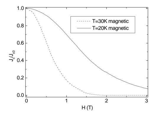
Figure 3: Field dependence of  $J_c$  for MgB<sub>2</sub>/Fe wire with perpendicular field. Dashed lines illustrate the anticipated field dependence of  $J_c$  at 24 and 32 K, when the effect of magnetic shielding is taken into account <sup>17</sup>.
