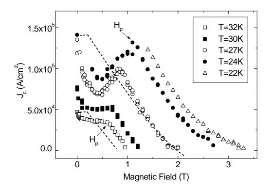
Figure 4: Temperature dependence of the field of the peak in the field dependence of  $J_c$ , for perpendicular field <sup>17</sup>. Solid and open symbols are for the nano-SiC doped and pure MgB<sub>2</sub>, respectively.
