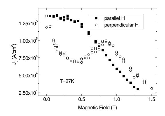
Figure 7: Comparison between the field dependence of  $J_c$  for parallel and perpendicular field <sup>17</sup>.
