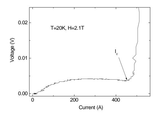
Figure 1: A typical voltage-current curve for  $MgB_2/Fe$  wire obtained by a pulsed current method <sup>17</sup>.
