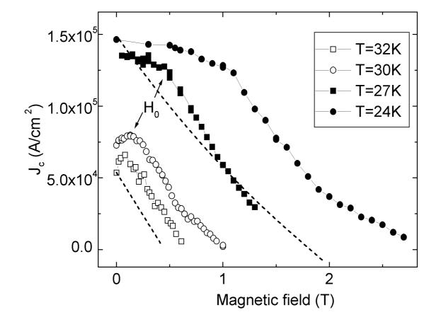
Figure 6: Temperature dependence of the field of transition from the plateau to decreasing regime in  $J_c$  vs. H, for parallel field <sup>17</sup>.
