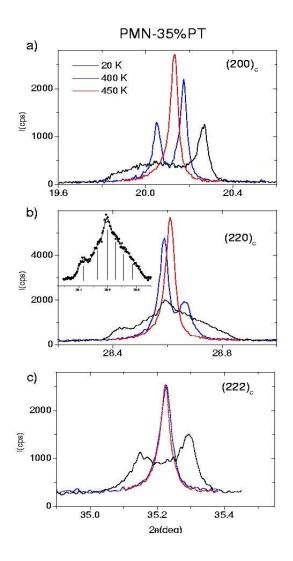
Fig. 2. X–ray scattering profiles of the (200) (220), and (222) Bragg reflections measured at 20, 400, and 450 K on a powder sample of PMN–35%PT. From Noheda *et al.* [5].
