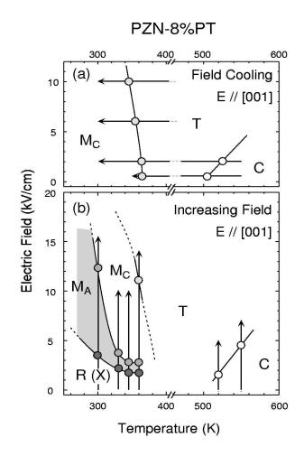
Fig. 9. Electric field versus temperature phase diagram for PZN–8PT. Data in (a) were obtained from field–cooled structural measurements. Data in (b) were obtained on increasing the electric field after ZFC (and ZFH for phase X). The arrows indicate both scan directions, and the ranges of the corresponding measurement sequences. Circles represent the transition temperatures and fields determined from each sequence. From Ohwada *et al.* [30].
