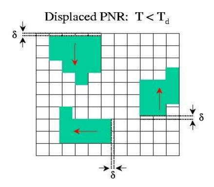
Fig. 5. A schematic representation of the polar nanoregions (shaded) surrounded by the undistorted cubic (white) lattice. The shift  $\delta$  is the same for all atoms within a given polar nanoregion, and is measured with respect to the cubic lattice.
