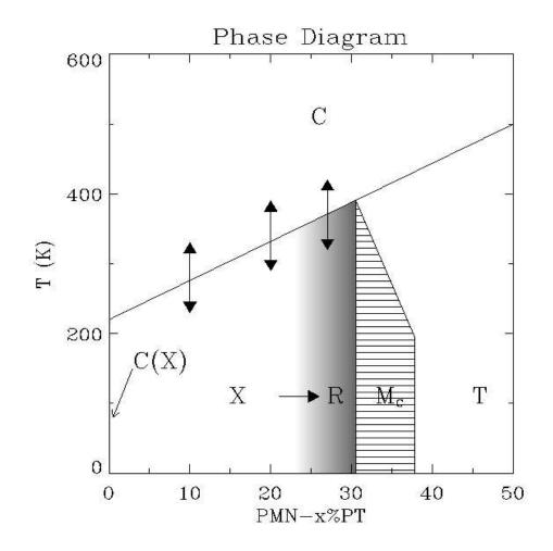
Fig. 8. The revised zero-field phase diagram of PMN-*x*PT. From Xu *et al.* [32].
