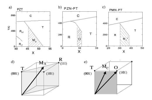
Fig. 1. Phase diagrams are shown for a) PZT, b) PZN–PT, and c) PMN–PT. The hatched regions indicate the  $M_A$  and  $M_C$  phases located near the MPB. From Noheda [6].
