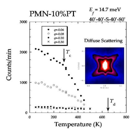
Fig. 4. Temperature dependence of the neutron diffuse scattering measured at  $\mathbf{Q} = (3,q,q)$  on a single crystal specimen of PMN–10PT. From Gehring *et al.* [18]. The inset shows a color contour map of the diffuse scattering around  $\mathbf{Q} = (1,0,0)$  in pure PMN as measured on the NIST Center for Neutron Research Disk Chopper Spectrometer at 300 K. From Xu *et al.* [19].
