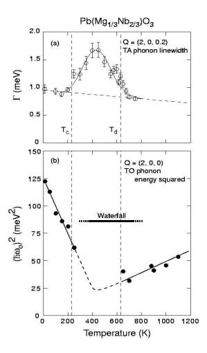
Fig. 3. (a) Plot of the intrinsic TA phonon linewidth  $\Gamma$  (open circles) versus temperature measured at  $\mathbf{Q} = (2,0,0.2)$ . Solid line is a guide to the eye. (b) Plot of the square of the zone center TO phonon energy versus temperature measured at  $\mathbf{Q} = (2,0,0)$ . The solid line is a fit to a linear temperature dependence, which is the hallmark of a ferroelectric soft mode. From Wakimoto *et al.* [17].
