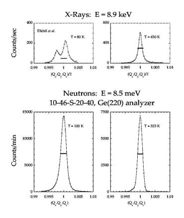
Fig. 7. Top panel: X–ray measurements of the (222) Bragg reflection in PMN–10PT by Dkhil et al. at 80 and 450 K [10]. Bottom panel: Neutron measurements of the (111) Bragg peak in single crystal PMN–10PT by Gehring et al. at 100 and 325 K [18]. The solid horizontal bar in each panel indicates the neutron spectrometer instrumental q–resolution FWHM.
