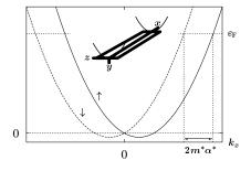
FIG. 1. Energy dispersion in the lowest spin split subband of a quantum wire. On the wire axis the spins  $s = \uparrow, \downarrow$  are polarized in the plane of the heterostructure parallel to the *z*-direction.
