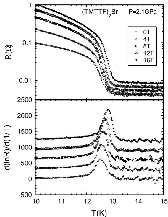
FIG. 3: Top: Temperature dependence of the resistance in  $(\text{TMTTF})_2\text{Br}$  for various magnetic fields at 2.1 GPa. Bottom: The derivative of the logarithm of the resistance by  $1/T$  offset from zero for clarity.
