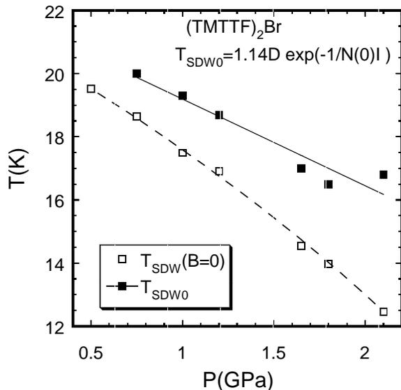
FIG. 2: Pressure dependence of the SDW transition temperature at zero magnetic field  $T_{\text{SDW}}(0)$  and the SDW transition temperature for the perfect nesting case  $T_{\text{SDW}0}$  estimated by fitting using the mean-field theory taking into account the magnetic-field dependence of the SDW transition temperature. The solid line is the best fit of the linear function. The dashed line is guide to the eye.
