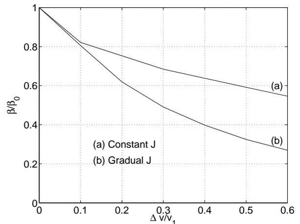
FIG. 3: Ratio of actual and ideal values of  $\beta$  as a function of the relative difference in velocities  $(v_2 - v_1)/v_1$  of the two electrons. The two qubits are assumed to enter the gate simultaneously and (a) completely from  $t = 0$  or (b) gradually.
