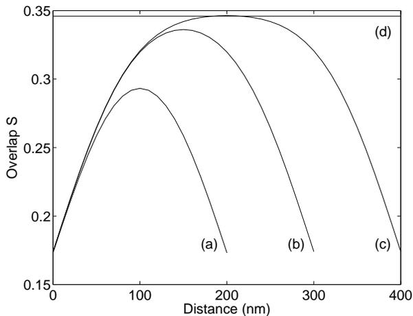
FIG. 1: The overlap  $S$  of two interacting orbitals as a function of the distance traveled along the gate. The qubits are allowed to enter the gate gradually and the gate lengths are (a) 200 nm, (b) 300 nm, (c) 400 nm. In (d) both qubits are assumed to enter the gate completely at  $t = 0$ . The two qubit gate was taken as perfectly symmetrical (*i.e.* electrons enter the gate simultaneously and with the same velocity).
