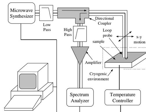
Fig. 1 System schematic. See Ref. [1] for details.
