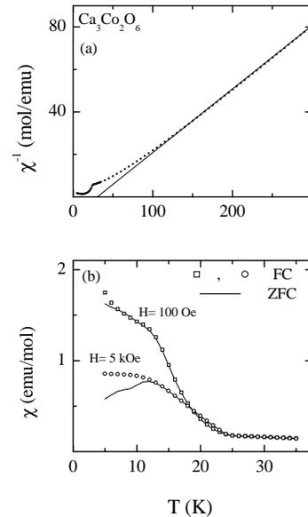
FIG. 2. (a) Inverse dc magnetic susceptibility ( $\chi$ ) as a function of temperature ( $T$ ) for zero-field-cooled  $\text{Ca}_3\text{Co}_2\text{O}_6$  measured in the presence of an external magnetic field ( $H$ ) 5 kOe. The line represent high-T linear region. (b) Dc  $\chi$  taken in the presence of 5 kOe and 100 Oe for zero-field-cooled (ZFC) and field-cooled (FC) states of the specimens are compared.
