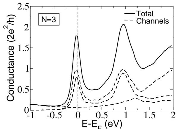
FIG. 3: Eigen-channel resolved conductance for the  $N = 3$  wire shown in Fig. 1. The two similar  $\pi$ -channels together with the  $\sigma$ -channel are indicated by the dashed lines, while the solid line shows the total conductance.
