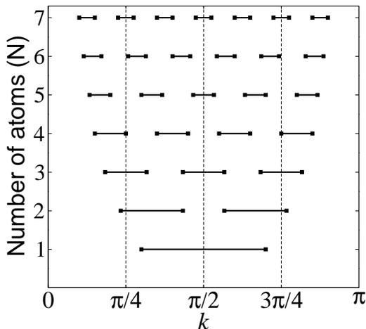
FIG. 4: Evolution in  $k$ -space of the discrete spectrum of a free  $N$ -atom wire. The interatomic distance in the wire is set to 1. The horizontal lines symbolize the width of the corresponding resonance formed when the free wire is coupled to electrodes.
