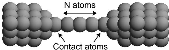
FIG. 1: The  $N = 3$  wire connecting Al(111) electrodes via a 3-atom basis. This structure constitutes the supercell in the DFT calculations and forms the scattering region in the conductance calculations.
