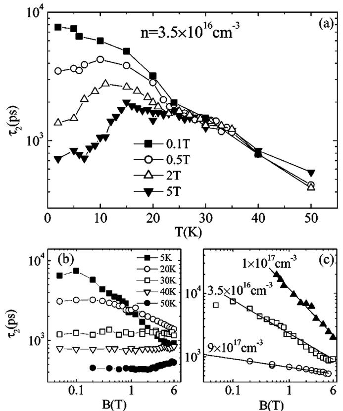
FIG. 9: Spin scattering time  $\tau_2$  of n-GaN at various magnetic fields (a), temperatures (b) ( $n = 3.5 \times 10^{16} \text{ cm}^{-3}$ ), and electron concentrations at 5 K (c) (after Beschoten *et al.* [57]).
