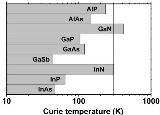
FIG. 1: Computed values of the Curie temperature for various p-type III-V compounds containing 5% of Mn in the  $S = 5/2$  high spin state and  $3.5 \times 10^{20}$  holes per  $\text{cm}^3$  (after [3, 4]).
