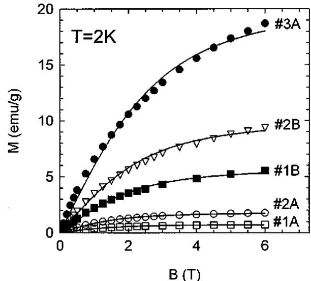
FIG. 5: Low temperature magnetization of  $\text{Ga}_{1-x}\text{Mn}_x\text{N}$  microcrystals (A) and bulk crystals (B) with  $0.0028 \leq x \leq 0.096$  showing paramagnetic behavior with weak antiferromagnetic spin-spin interactions (after Zajac *et al.* [41]).
