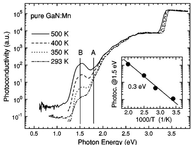
FIG. 3: Temperature dependence of photoconductivity spectra of GaN:Mn. The absorption, whose onset is marked by A, is interpreted as photoionization of the Mn acceptor-like state. The temperature dependent peak B is interpreted as acceptor photoionization process involving internal transitions within the Mn ions and thermally activated process characterized by an activation energy  $E_A \approx 0.3$  eV (after Graf *et al.* [9]).
