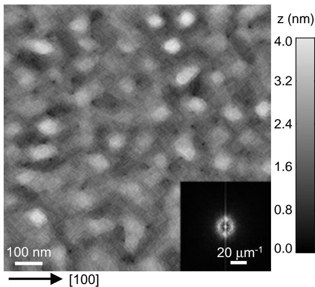
FIG. 1: STM image of a  $\text{Si}_{0.7}\text{Ge}_{0.3}$  layer, 3.8 nm thick, grown on Si(001) at a substrate temperature of  $600^\circ\text{C}$  and annealed for 20 s. Inset: average Fourier transform of six similar images. The observed ring corresponds to an average distance of 125 nm between mounds.
