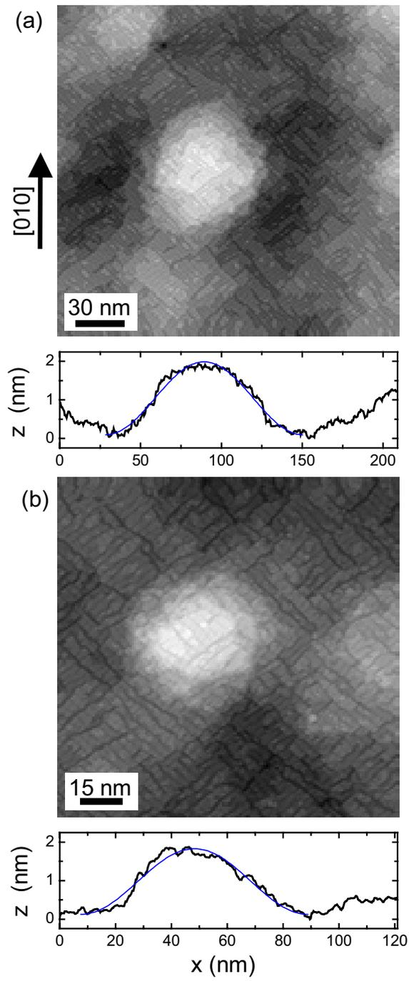
FIG. 2: STM images of  $\text{Si}_{0.7}\text{Ge}_{0.3}$  (a) and  $\text{Si}_{0.5}\text{Ge}_{0.5}$  (b) prepyramids and corresponding line scans through the center of the islands. Cosine fits of the line scans are also shown.
