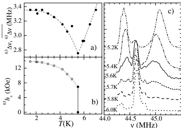
FIG. 3: (a) Uniform frequency shift for the  $^{63}\text{Cu}$  central transition. The line is a guide to the eye. (b) The staggered hyperfine field obtained from the splitting of the  $^{63}\text{Cu}$  central line. At 5.5 K, the spectrum consists of unsplit ( $^{63}h_s = 0$ ) and split (finite  $^{63}h_s$ ) lines. (c) Evolution of the high-frequency satellite  $^{35}\text{Cl}$  NMR spectrum across the phase boundary. All data were taken at  $H = 8.56$  T.
