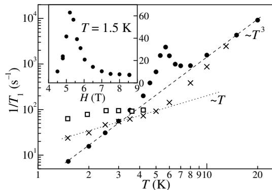
FIG. 5: Temperature dependence of  $^{63}\text{Cu}$  spin-lattice relaxation rate at  $H = 5.2$  T (squares), 4.8 T (crosses), and 8.5 T (circles). Inset: Field dependence of the relaxation rate at 1.5 K.
