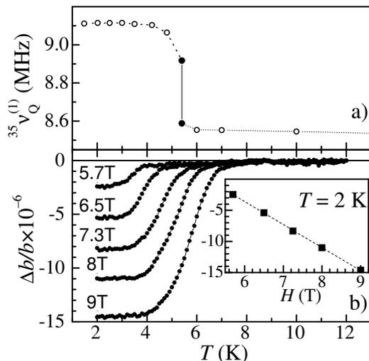
FIG. 4: (a) First-order quadrupole shift for  $^{35}\text{Cl}$  extracted with eq. (3) from the data in Fig. 2(b). (b)  $b$ -axis thermal expansion in different magnetic fields. The insert shows the  $b$ -axis strain *versus* magnetic field at 2 K.
