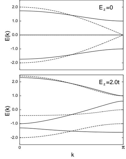
FIG. 15: Electron dispersion for the zigzag chain of the CE phase (solid lines) and for the linear chain of the C phase (dashed lines) calculated for different crystal-field splittings in the  $\{|x\rangle, |z\rangle\}$  orbital basis at corner sites ( $E_z$ ). The orbitals at the bridge sites are degenerate (assuming  $\eta = 0$ ).
