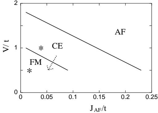
FIG. 11: Phase diagram as in Fig. 2 including the local nearest- and next-neighbor OO interactions with  $\kappa = 0.2t$  and  $\kappa' = 0.1t$  (spring constants  $K_2/K_1 = 0.25$ ). '\*' indicate representative points in the CE region for which the correlation functions are presented here. The dashed arrow presents the direction of the transition from the localized CE to the itinerant electron A-phase at low temperatures.
