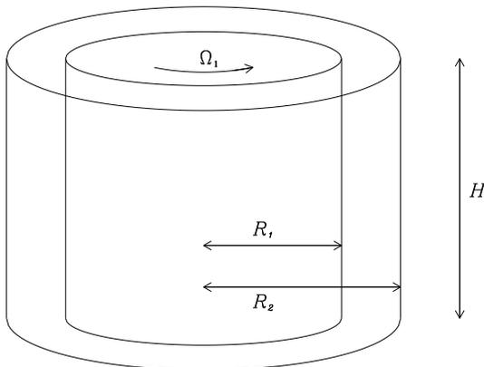
FIGURE 1. The problem's configuration. The fluid is contained inside a cylindrical box of inner radius  $R_1$ , outer radius  $R_2$  and height  $H$ . The inner cylinder rotates at constant angular velocity  $\Omega_1$ , while the outer cylinder and the top and bottom end plate are stationary.
