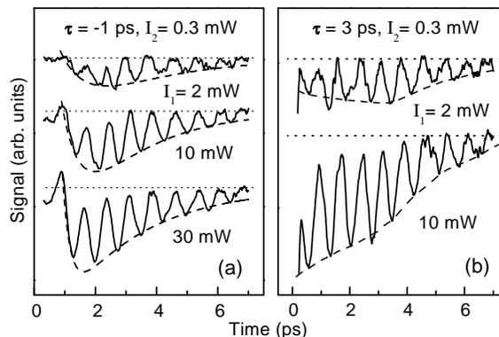
FIG. 3: Time evolution of the TR-PPDR signal (solid lines) at a few pump intensities ( $I_1$ ) at  $\tau = -1$  ps (a) and 3 ps (b), with  $I_2 = 0.3$  mW. The signal is  $-ve$  and the data for different  $\tau$  are shifted along the vertical axis (linear scale), with the zero of the signal shown as dotted lines. The dashed lines are shown as the envelope of the signal to guide the eye.
