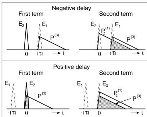
FIG. 4: Schematic representation of the origin of the TR-PPDR signal due to the two terms in Eq. (2) at  $-ve$  (upper panel) and  $+ve$  (lower panel) delay. The shaded regions indicate the time domain in which the TR-PPDR signal arises due to overlap of  $\mathcal{P}^{(3)}(t)$  in  $t$  with  $\mathcal{E}_2(t)$  (first term) and  $\mathcal{P}_2^{(1)}(t)$  (second term).
