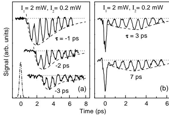
FIG. 2: Time evolution of the TR-PPDR signal (solid lines) at a few  $-ve$  (a) and  $+ve$  (b) delays are shown on linear scales. Here pump (probe) intensity  $I_1$  ( $I_2$ ) = 2 (0.2) mW. The signal is  $-ve$  and the data for different  $\tau$  are shifted along the vertical axis, with the zero of the signal shown as dotted lines. The dashed lines are shown as the envelope of the signal to guide the eye. The cross-correlation trace for the probe pulse is plotted in (a) (dashed-dotted line).
