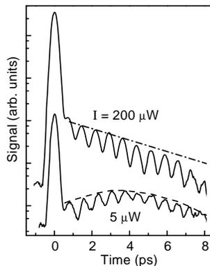
FIG. 6: Semilogarithmic plot showing the time profile of the coherent emission along the probe reflection direction (no pump pulse) for two average intensities ( $I = 200$  and  $5 \mu\text{W}$ ) of the incident pulse. Data at two  $I$  are shifted vertically. The dash-dotted line is an exponential fit, the dashed curve is drawn to guide the eye.
