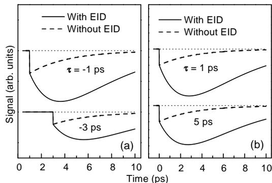
FIG. 5: Simulation of TR-PPDR signal using Eq. (2) calculated within optical Bloch equation for  $\delta$ -like electric fields for  $-ve$  (a) and  $+ve$  (b) delays, highlighting the role of excitation induced dephasing (EID). The signal is  $-ve$  and the curves for different  $\tau$  are shifted along the vertical axis (linear scale), with the zero of the signal shown as dotted lines.
