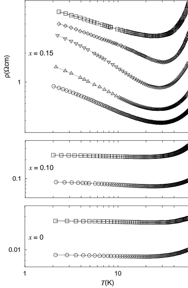
Fig. 2. Log-log plot of the low-temperature resistivity for all samples. The highest curve of each set (squares) is the zero-field result. The lowest curve of each set (circles) corresponds to  $\mu_0 H = 9$  T. The intermediate curves for  $x = 0.15$  correspond to  $\mu_0 H = 1, 3,$  and  $6$  T, respectively from top to bottom. The lines joining the points are just guides for the eye.
