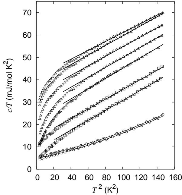
Fig. 1. Specific heat measurements for  $x = 0.15$  (upper set { triangles),  $0.10$  (middle set { squares), and  $0$  (bottom set { circles). The highest and lowest curves of each set correspond to zero applied field and to  $\mu_0 H = 9$  T, respectively. The intermediate curves for  $x = 0.15$  correspond to  $\mu_0 H = 1, 3,$  and  $6$  T, respectively from top to bottom. The solid lines are fittings to Eqs. (1) or (2).
