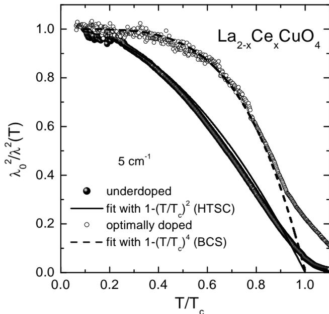
FIG. 3: Temperature dependence of the penetration depth in optimally doped ( $x = 0.106$ ,  $T_c = 30$  K) and underdoped ( $x = 0.081$ ,  $T_c = 25$  K)  $\text{La}_{2-x}\text{Ce}_x\text{CuO}_4$  at  $5 \text{ cm}^{-1}$ . Points - experimental data, lines indicate fits using  $1 - (T/T_c)^2$  (solid) and  $1 - (T/T_c)^4$  (dashed).
