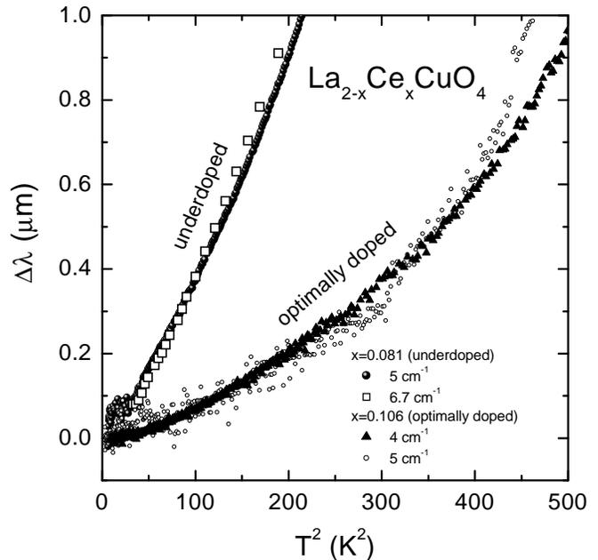
FIG. 4: Temperature variation of the penetration depth in  $\text{La}_{2-x}\text{Ce}_x\text{CuO}_4$  at low temperatures *vs.*  $T^2$ . The experimental data for  $\nu = 5 \text{ cm}^{-1}$  are replotted from Fig. 3, two additional data sets at 4 and  $6.7 \text{ cm}^{-1}$  are added for the optimally doped and the underdoped samples, respectively.
