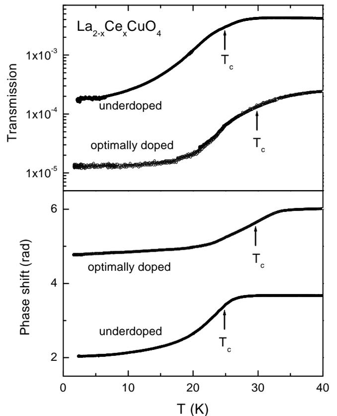
FIG. 2: Temperature dependence of the millimeter-wave ( $5\text{ cm}^{-1}$ ) intensity transmission (top panel) and of the corresponding phase shift (bottom panel) for optimally doped ( $x = 0.106$ ,  $T_c = 30$  K) and underdoped ( $x = 0.081$ ,  $T_c = 25$  K)  $\text{La}_{2-x}\text{Ce}_x\text{CuO}_4$  films on  $\text{SrLaAlO}_4$  substrates.
