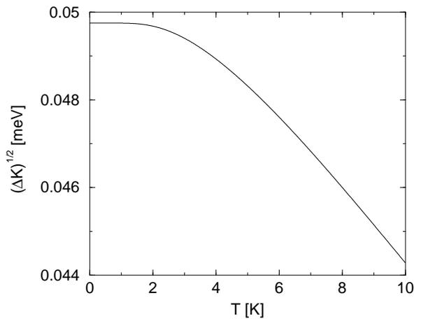
FIG. 1: Temperature dependence of the gap  $\sqrt{\Delta K}$ .
